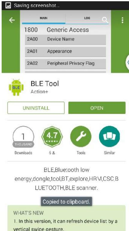
7.2.6.9 After the installation is complete, open the app. After the application opens and scans, you should see at least one entry for ARROW BLE WIFI CAPE. Note the negative number on the left side of each entry. This is the device's Received Signal Strength Indicator (RSSI) number. It measures the strength of the Bluetooth device's signal in dB.
