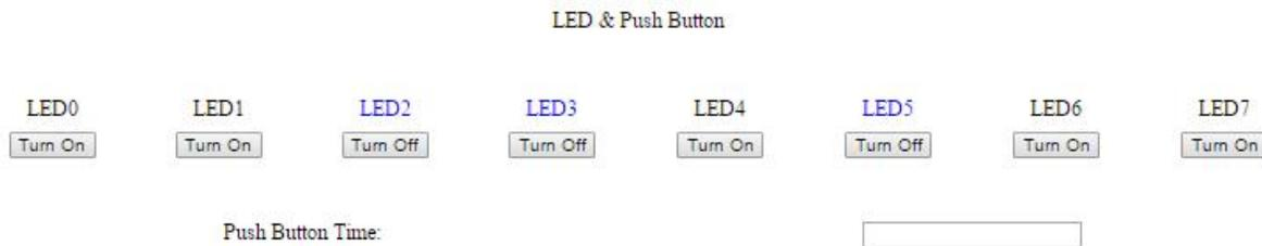
Click a few LED buttons in the webpage and observe the corresponding LEDs illuminating on the DECA board.
