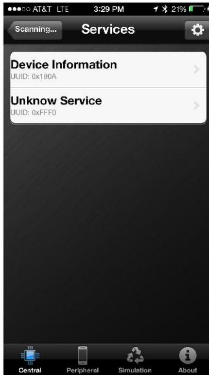
The CC2650 has been configured to provide two data "services". One provides Device Information such as system ID, hardware revision, and serial number; each of these fields is called a "characteristic". The other, titled "Unknown Service", allows the BLE Utility app to read temperature, humidity, and accelerometer data from the DECA board.
