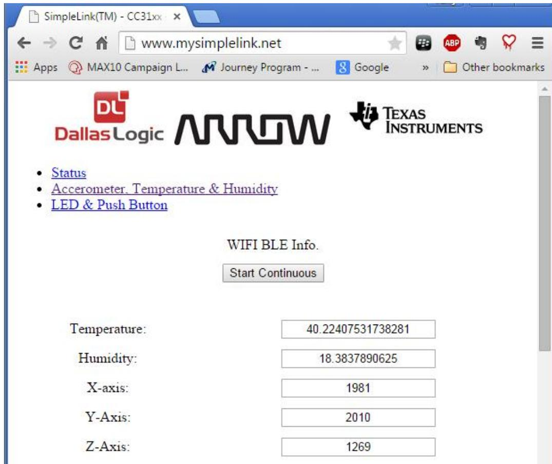
Tilt the DECA board in various directions to see if you can determine the X, Y and Z orientations of the board.
