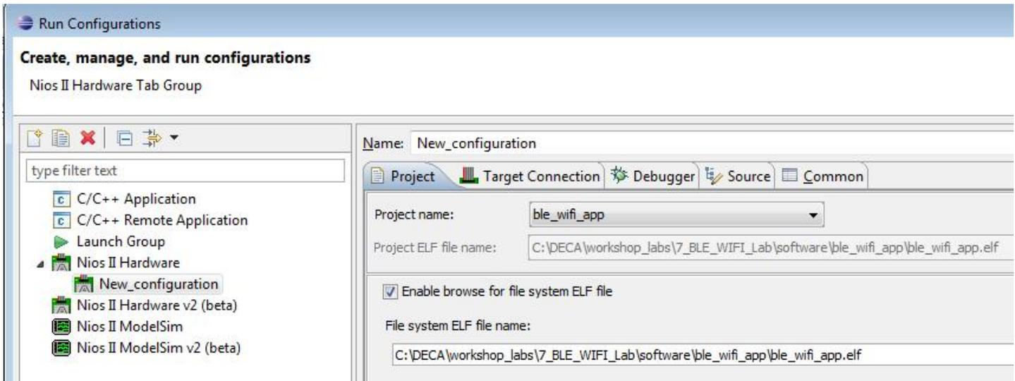
7.2.4.8 In the Target Connection tab, click the Refresh Connections if the Run button has been grayed out.
